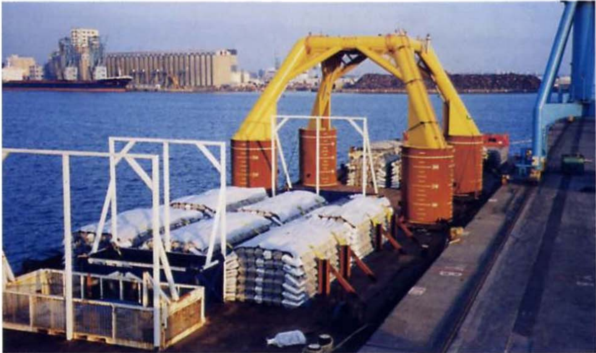
Sea fastenings used to secure concrete mats and a float onto a barge.
