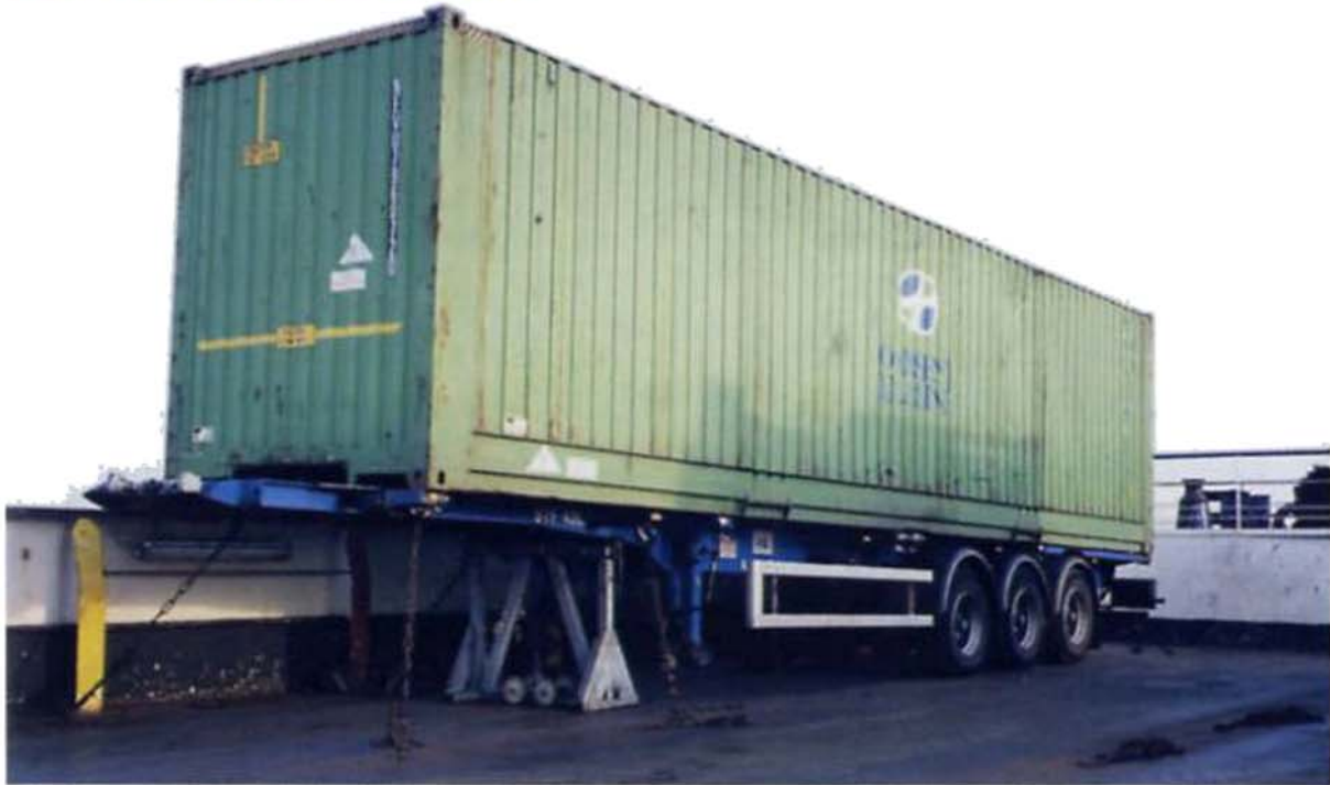
Ro-ro container trailer secured on trestle
