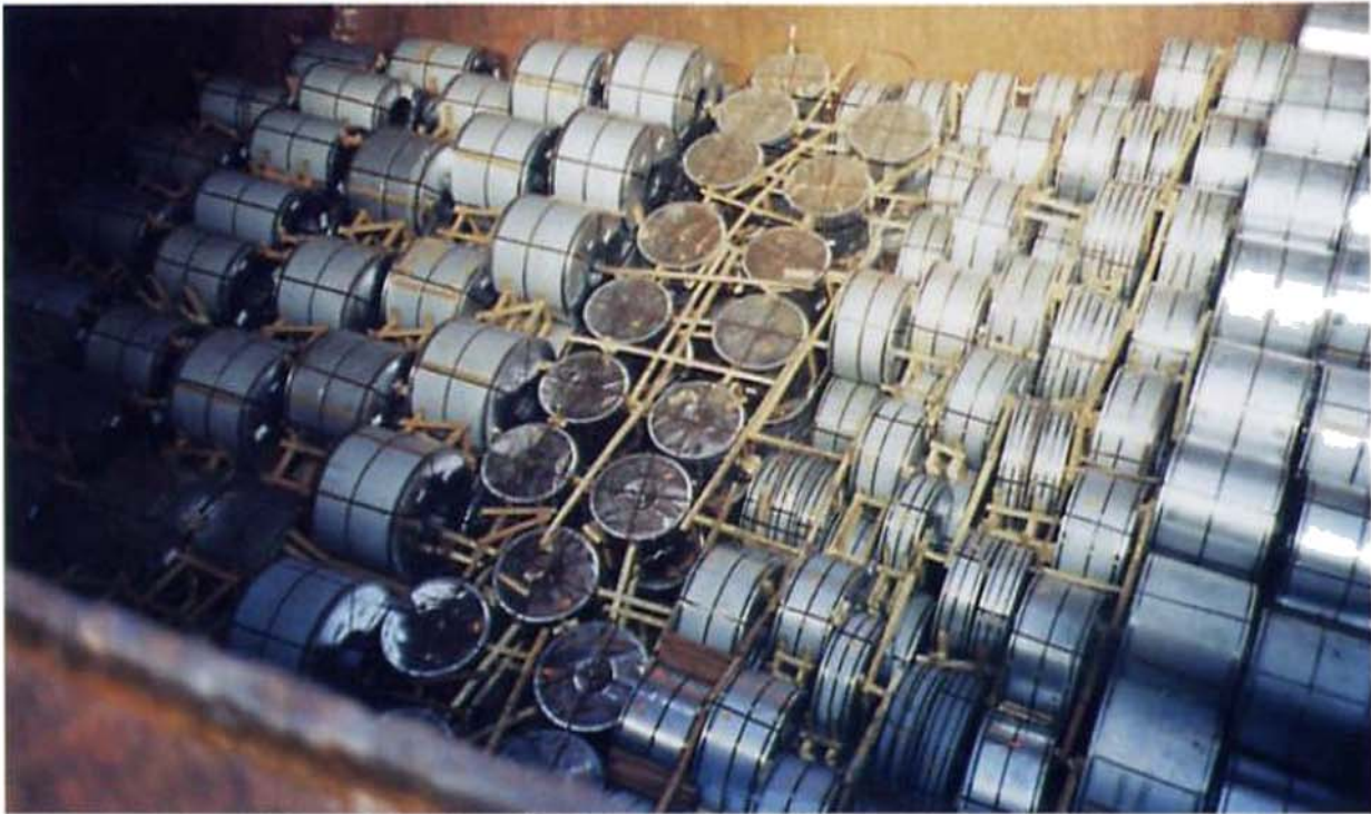
Steel products being stowed in the hold of a bulk carrier.
