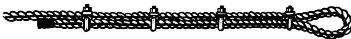
An eye in a wire rope properly made up using 4 grips.
