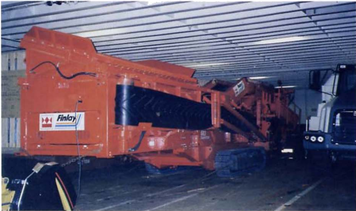
Tracked vehicle secured on vehicle deck
