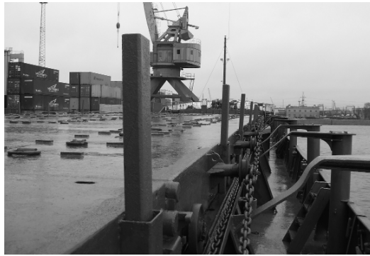
Figure 6.7. Example of uprights for bottom blocking
