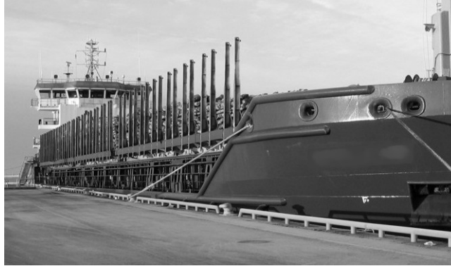
Figure 6.9. Uprights for blocking over the entire height of the stow
