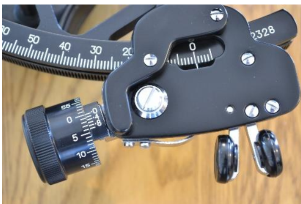
Fig. 1 - With sextant set at exactly 0^{\circ} 00.0' the horizon should appear as a continuous straight line.
