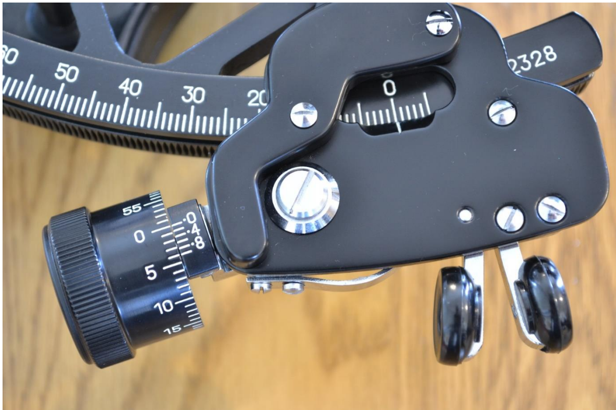
Fig. 4 - When the sextant is set at exactly zero the Index Mirror and Horizon Mirror should be parallel to each other.
